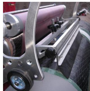
4.step: application of the pcw (permanent carbon wrap) with pcw -winder
